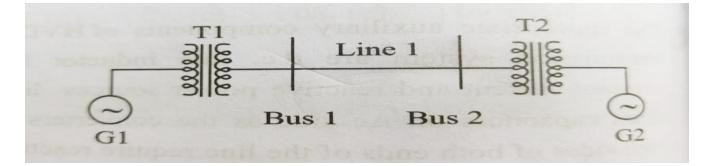
Choose 25 KV as the base voltage at the generator G1 and 200 MVA as the MVA base.
