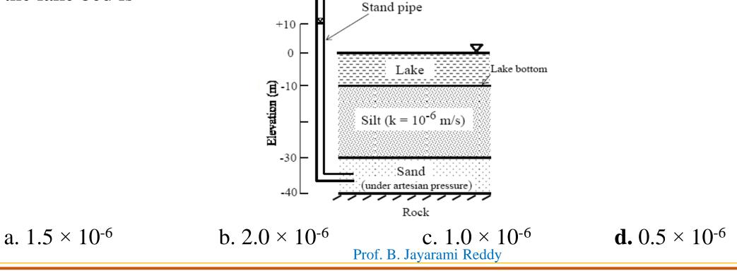
8 Ans. d Coefficient of permeability of silt,  $k = 10^{-6} m/s$ Stand pipe Total head, H = 10m+100 Length of silt layer, L = 20mLake lake bottom Hydraulic gradient,  $i = \frac{H}{L} = \frac{10}{20} = 0.5$ Elevation (m) Silt (k =  $10^{-6}$  m/s) Area of sand layer =1 unit Quantity of water flowing into lake through -30 Sand silt layer, (under artesian pressure) -40 L Rock
