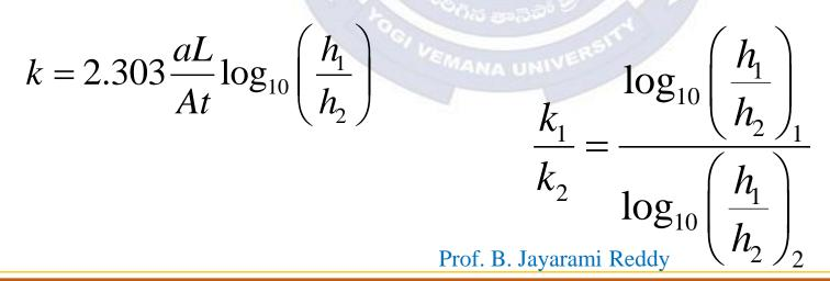
$$\left(\frac{h_{1}}{h_{2}}\right)_{1} = 1.25 \quad ; \quad k_{2} = 5k_{1} \quad ; \quad \left(\frac{h_{1}}{h_{2}}\right)_{2} = ?$$
