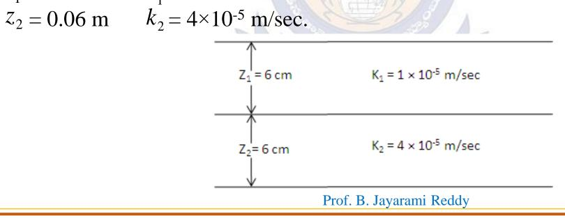
Length of the sample, L = 12 cmCross sectional area of sample = 50 cm<sup>2</sup>. Initial head,  $h_1 = 40 \text{ cm}$ Final head,  $h_2 = 20 \text{ cm}$ Time taken to fall from  $h_1$  to  $h_2 = ?$ Cross sectional area of stand pipe,  $a = 2 \text{ cm}^2$ . Average permeability perpendicular to the bedding planes,
