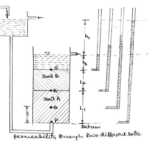
Pressure head = Height of water column in piezometer
