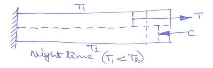
During the day, the top of the pavement slab gets heated under the sunlight when the bottom of the slab still remains relatively colder. Due to frictional resistance, tensile stresses induced at bottom during the day. During the night (or late in the evening), the bottom of the slab gets heated up due to heat transfer from the top. Due to frictional resistance, compressive stress induced at the bottom during the night. Therefore, it can be concluded that
